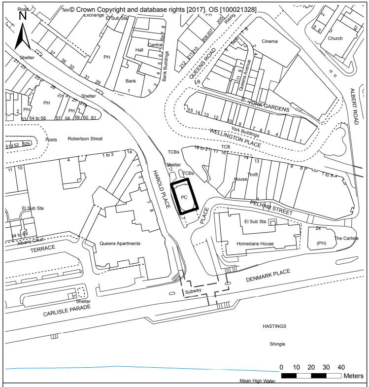
Public Conveniences Harold Place Hastings TN34 1JA Demolish the existing redundant local authority public convenience root and superstructure complete down to ground floor slab level and finish the resulting flat pedestrian area with pre-cast concrete paving slabs with an appearance complimentary to the surrounding pedestrianised town centre surface finishes. The existing basement level service directly void beneath the superstructure is to be retained.
